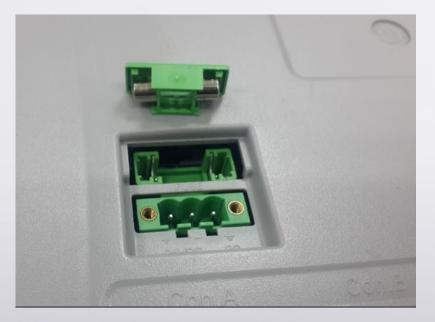
*Step 3.* Put the fuse holder back to its original place.
