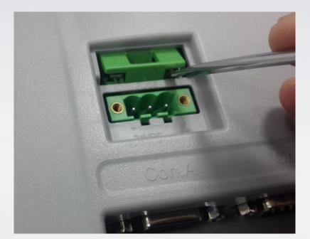
*Step 2.* Remove the blown fuse and replace with a right one for the
